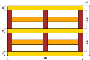
Nails/Joint: Deck board/Block 2 pcs. 3.1/85 mm ring nail
