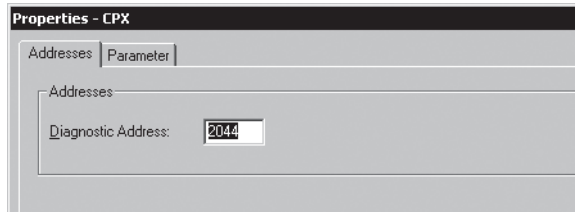
Fig. 2/12: Changing the diagnostics address with Siemens STEP 7 – HW Config
