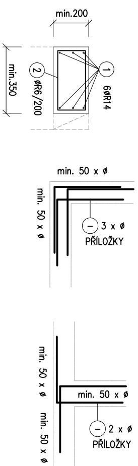
**SCHÉMA VYVÁZÁNÍ ROHŮ A "T" SPOJENÍ**
