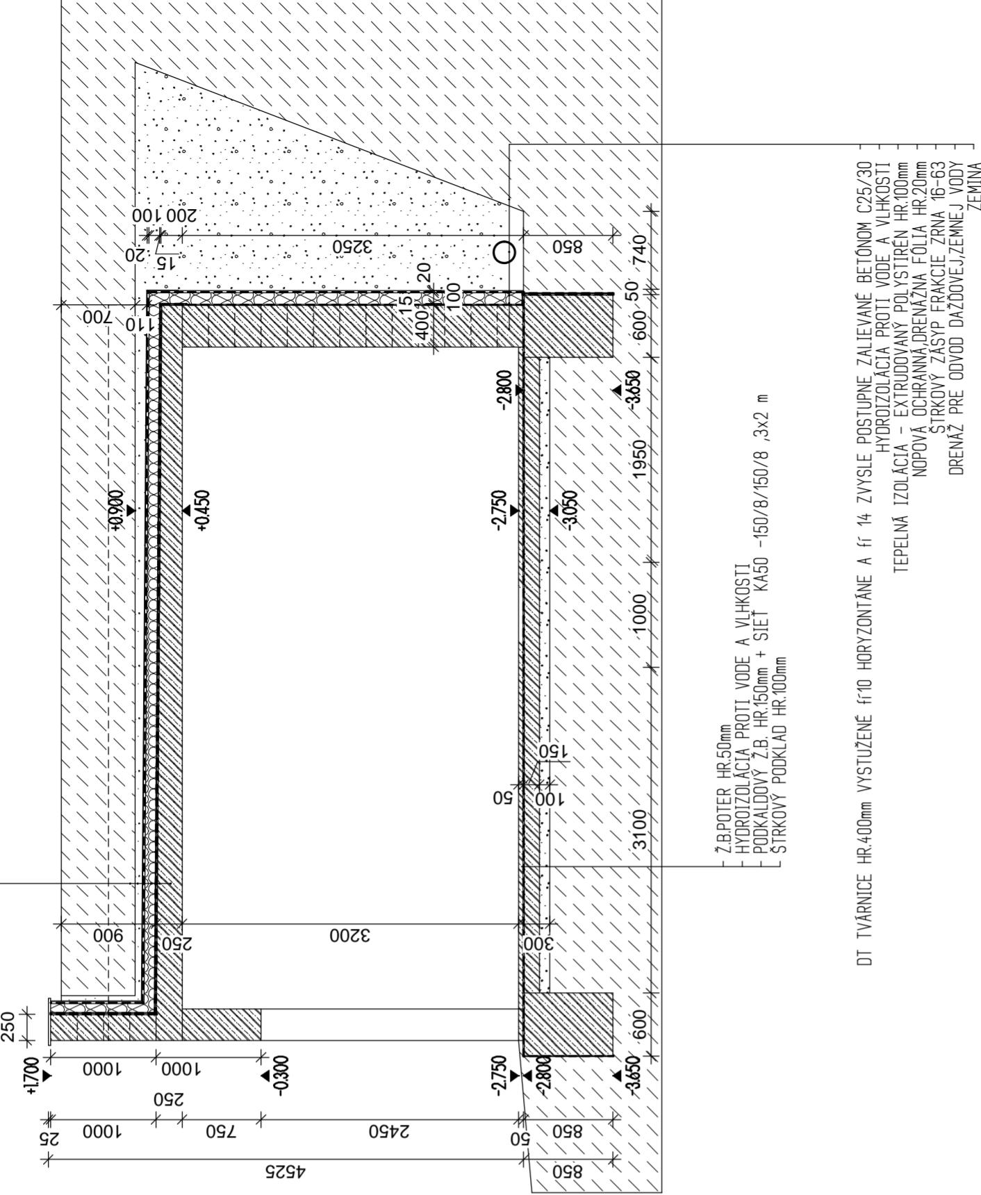
DT TVÁRNICE HR.400mm VYSTUŽENÉ fí10 HORYZONTÁNE A fí 14 ZVÝSLE POSTUPNE ZALIEVANÉ BÉTONOM C25/30 HYDROIZOLÁCIA PROTI VODE A VLIKOSTI TEPEĽNÁ IZOLÁCIA - EXTRUDOVANÝ POLYSTIREN HR.100mm NOPOVÁ OCHRANNÁ DRENÁZNA FOLIA HR.20mm ŠTRKOVÝ ZASYP FRAKCIE ZRNA 16-63 DRENÁZ PRE ODVOD DAŽDOVEJ,ZEMNEJ VODY
