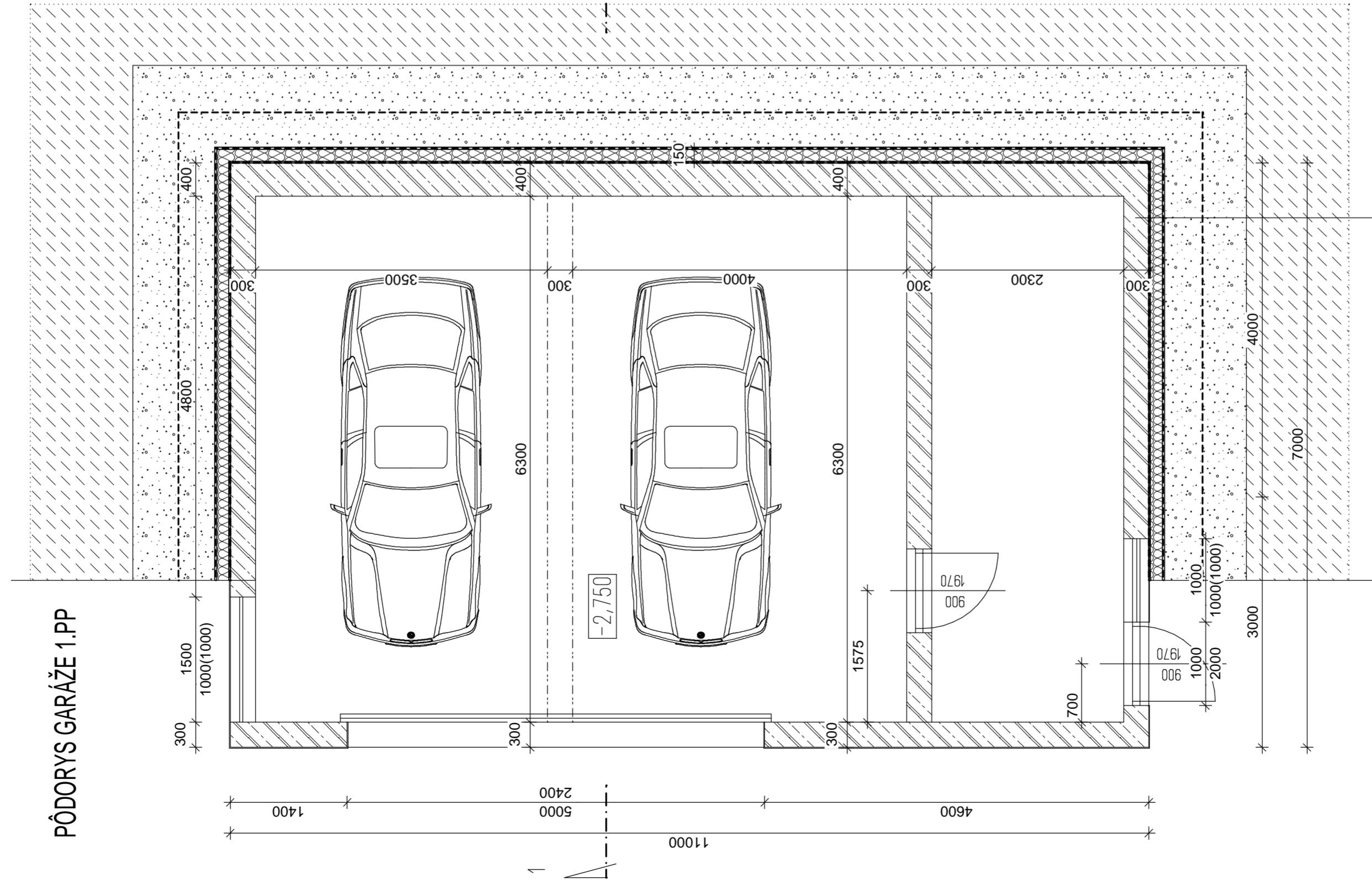
DT TVÁRNICE HR.400mm VYSTUŽENÉ ff10 HORYZONTÁNE A ff 14 ZVÝSLE POSTUPNE ZALIEVANÉ BÉTONOM C25/30
