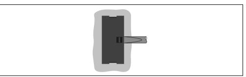
Figure 59: CP340, CP360, CP380 and CP382 - removing the cover for the lithium battery
