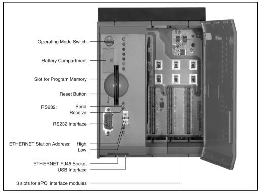
Figure 58: CP382 operational and connection elements
